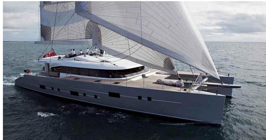
mousetrap - 110' Catamaran - VPLP110 Carbon hulls & superstructure
