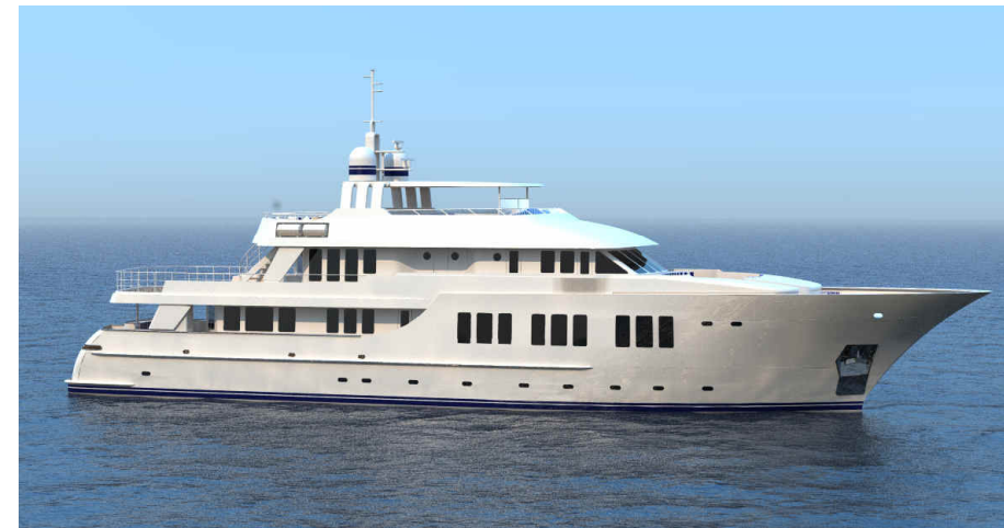
135' Motor Yacht - Steel hull and Aluminium superstructure
