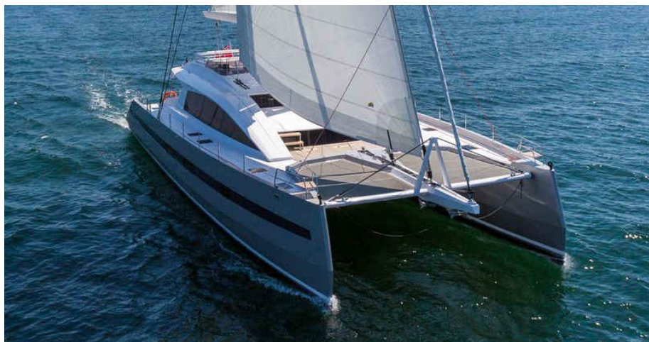
WindQuest - Long Island 85' n°1 Catamaran Aluminium hulls & composite superstructure
