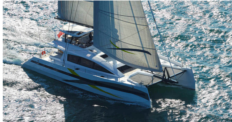
NDS Evolution - Long Island 85' n°2 Aluminium hulls & composite superstructure
