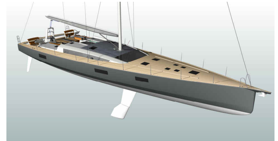
70' Fast Cruising Sloop Aluminium hull & composite superstructure
