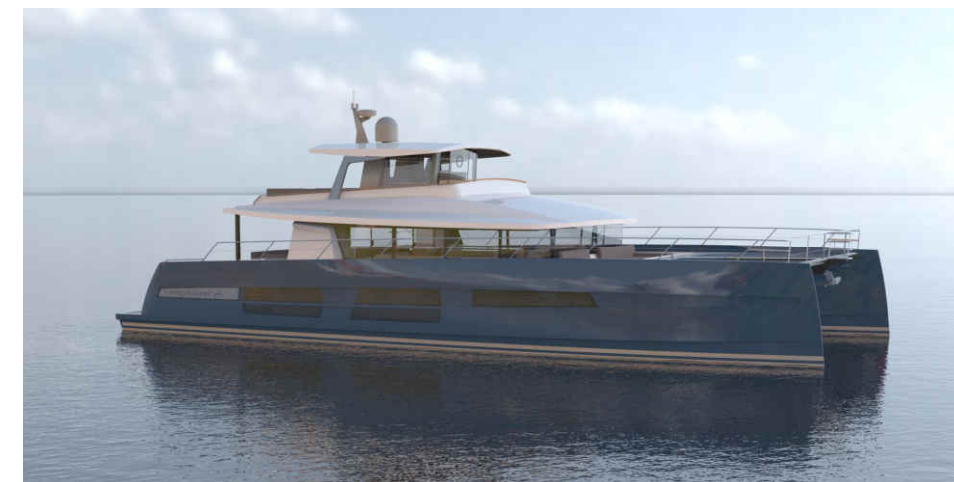
Long Island 78' Power Aluminium hull & composite superstructure
